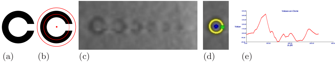
Fig. 3. (a) LR with gap on the right side. (b) Marked features: center of ring (dot), path inside the ring (line), path in the gap (dotted line) and circle-path outside (line). (c) LRs on Step 7, Exposure 99 mAs, Barzilai Borwein reconstruction, TV \lambda = 0.5 . (d) Visual output of the automatic LR detection for the first Ring in (c): center, ring and gap are marked correctly. (e) Values on the circle-path through the ring and the gap: the highest peak belongs to the gap.
